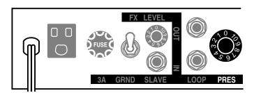
Control compress the sound and enhance the more vocal like qualities of single notes. This control can also produce a fatter, warmer character, especially when lead style sounds are dialed up on the **MARK I**. Lower Treble settings, combined with low Presence settings produce the richest, roundest lead sounds.
